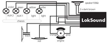
Figure 3: Wiring of engines with DC motors and functions with the common pole connected to the chassis
