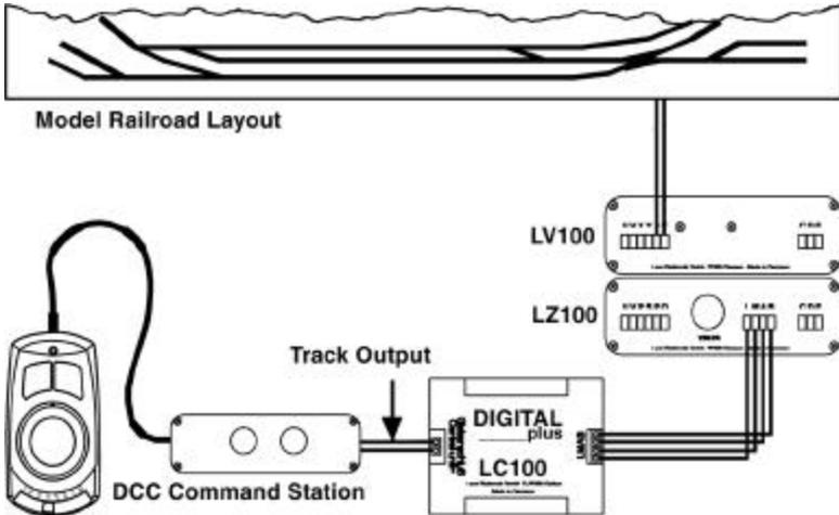
Figure 1 Connecting the LC100 to a ROCO "Digital is Cool" or LGB "Multi Train Control" DCC System
