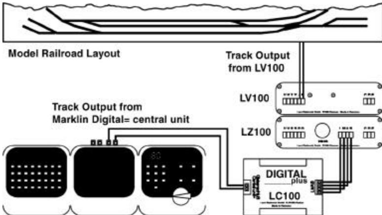
Figure 2 Connecting the Arnold or Märklin Digital= system to the LC100
