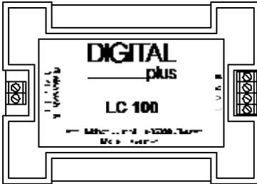
The XpressNET DCC Converter LC100 connects input devices from other manufacturer's NMRA DCC systems with any XpressNET based system. This allows reuse or expansion of other systems with DIGITAL plus.
