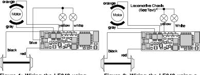
Figure 1: Wiring the LE040 using floating common
