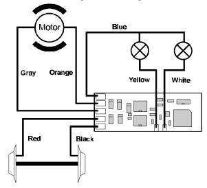
Figure 2: Wiring the LE103XF using a floating common.
