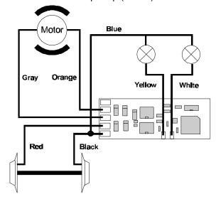
Figure 1: Wiring the LE103XF using track voltage common
