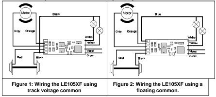
Place the locomotive (without the body) on the programming track and read back the locomotive's address from the decoder. If the decoder is properly installed, you will be able to read back the factory pre-set address 03. Remove the locomotive from the track, and if necessary correct any wiring errors.
