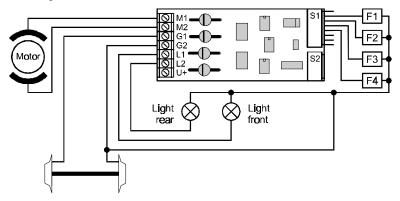
Figure 1: Wiring the LE230 using track voltage common
