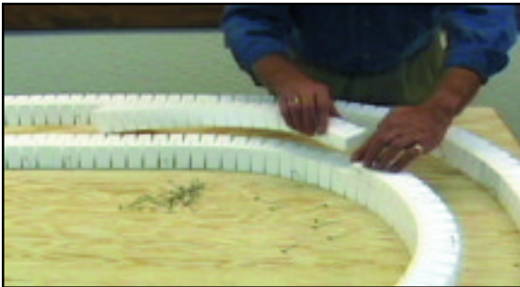
Center the Inclines on top of the Risers and pin them in place with Foam Nails.
