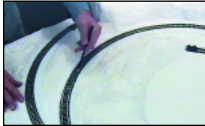
When satisfied with position of track, trace outline onto the Plaster Cloth hardshell.
