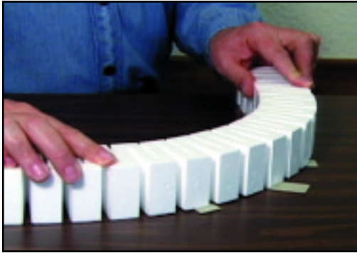
For banking the shims need to be inserted under the outside of curves before gluing in place.
