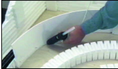
After flexing, 1/4" Foam Sheets work great for curves. Pin in place with Foam Nails and glue in place with the Low Temp Foam Glue Gun.
