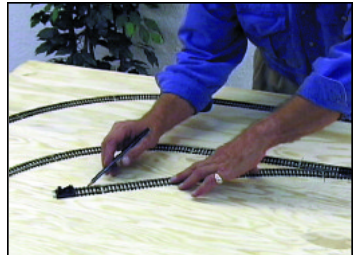
Trace a line around both sides of your track directly on the plywood base.
