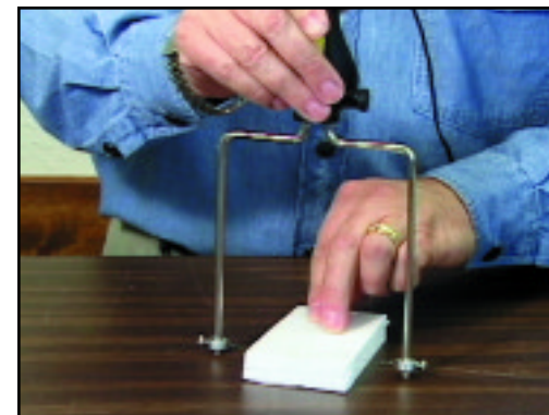
Adjust height of wire and push foam through the cutter for exact thicknesses.
