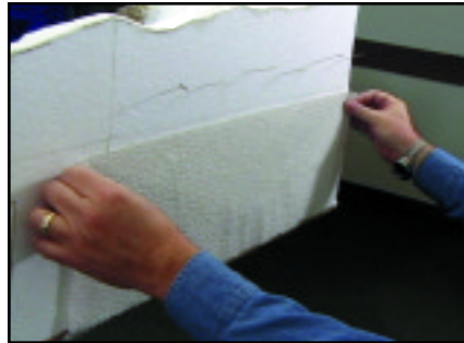
Plaster Cloth can be used to create a hardshell on the exterior surface of the Profile Boards.
