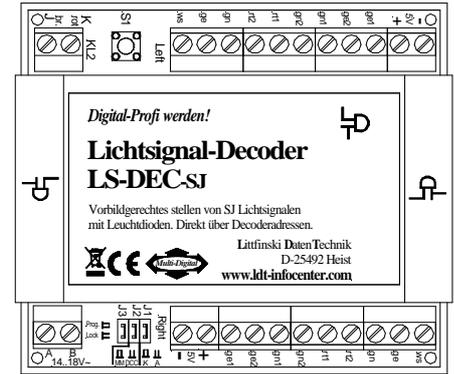
The decoder receives the **power supply** via the two poles clamp **KL1**. The voltage shall be within a range of 14..18V~ (alternate voltage output of a model rail road transformer).
