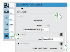
You can adjust the status query interval if necessary in the information and settings segments. Tap on the plus symbol in the "Locomotives" segment in order to add locomotives. Select with a tap of your finger in the selection window that is turned on (small image). Locomotives that have been added will appear after that in the lowest position (left image).
