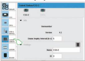
You can assign an individual designation in the Central Station settings. Moreover, you can set the interval of how frequently the device's status is queried. Standard setting: every five seconds. The ID is automatically assigned. In the case of a new device replacing a defective device, enter the value here for the old device.
