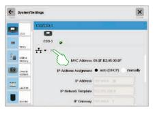
You must first find out the IP address for your CS3 in order to start the Web interface. To do this call up the CS3 system settings (see Page 32) and there open the section "IP". In the standard setting, the CS3 automatically receives an IP address assigned to it from the router connected to it. This is shown in the field "IP Address" (left image).
