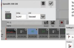
You can enter corresponding time units in the delay field in order to have procedures match each other exactly in terms of time. The delay indicates here when the next event is to be activated.
