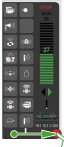
Pull the red circle with a small white locomotive in the direction of the center of the screen: The locomotive functions become visible, eight functions per column. Up to 32 functions can be shown at a time depending on how far you pull the list up.
