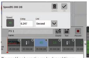
This is the way adjusting settings works: Call up the item "Edit event" and tap on the corresponding procedure. The event changes to the editing mode, recognizable from small "x" signs in the squares above right.
