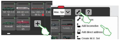
Locomotives without an mfx decoder are added by hand. To do this simply tap on the large plus sign at the end of the locomotive list. You can also tap on the tool symbol ("Edit") in the locomotive list and select ..Add locomotive" in the menu that is turned on.
