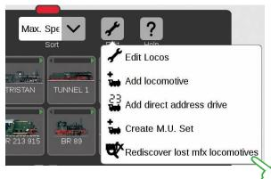
In rare cases, it can happen that an mfx locomotive is no longer displayed in the locomotive list. This option can be helpful. All of the existing data are checked and the system investigates for missing mfx locomotives.
